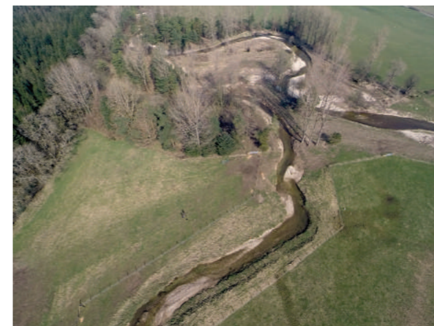
Figure 5.11 (Left) Aerial view of the River Lyvennet and Howe Beck, Cumbria in Autumn 2014 after re-meandering and diversion from the previously channelised rivers resulting in nearly 2 km of new river habitat (© Oliver Southgate, Environment Agency). (Right) The Howe Beck nine months after excavation and diversion along the course of an old channel (© Daniel Brazier, Eden Rivers Trust).
