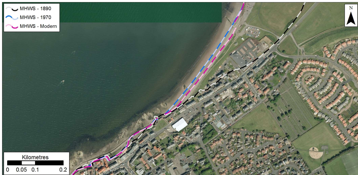
Figure 1.15: MHWS position in 1890, 1970s, and Modern datasets at Prestonpans. Getmapping are our current providers of Scotland-wide digital aerial imagery© Getmapping plc.
