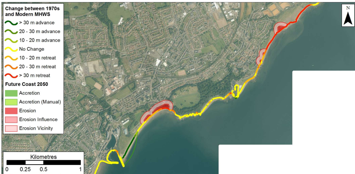
Figure 1.24: Possible future coastline position in 2050 based on rates between 1970 and Modern MHWS data in Dysart. Getmapping are our current providers of Scotland-wide digital aerial imagery© Getmapping plc.
