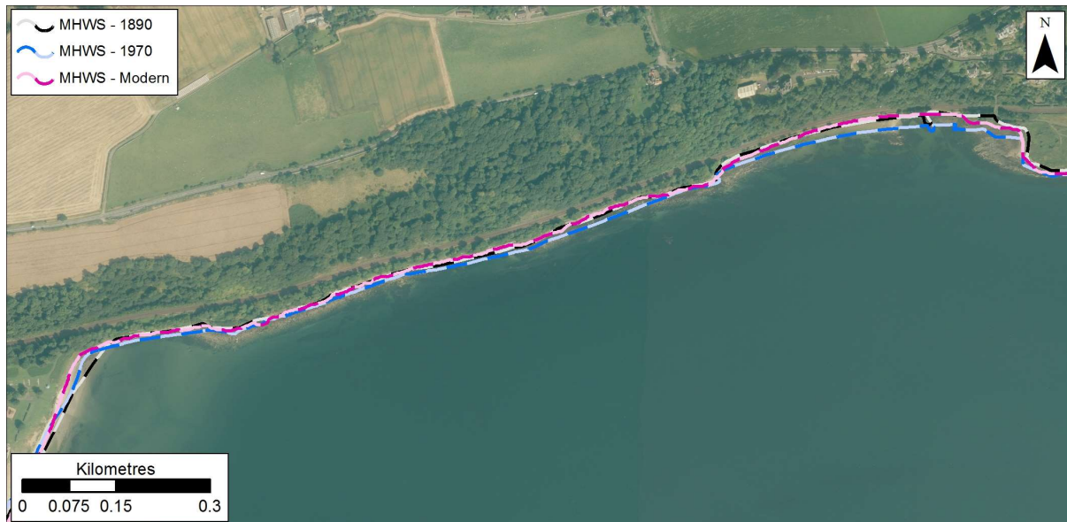
Figure 1.20: MHWs position in 1890, 1970s, and Modern datasets at Aberdour and Burntisland. Getmapping are our current providers of Scotland-wide digital aerial imagery © Getmapping plc.
