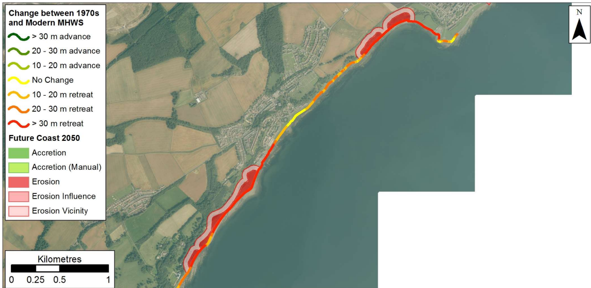
Figure 1.27: Possible future coastline position in 2050 based on rates between 1970 and Modern MHWS data at East Wemyss. Getmapping are our current providers of Scotland-wide digital aerial imagery© Getmapping plc.
