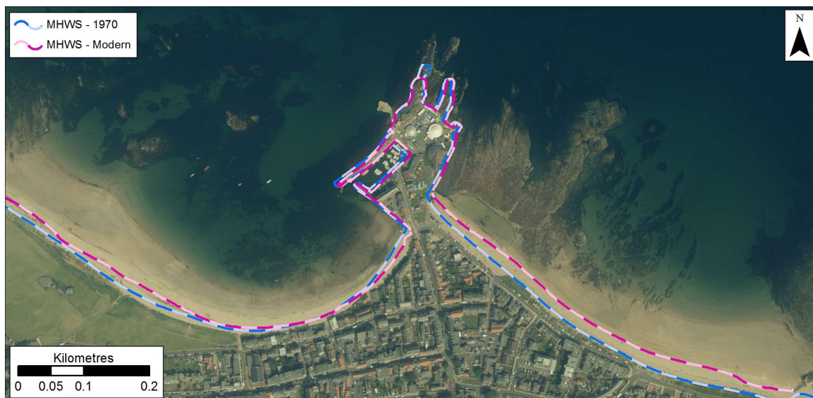
Figure 1.8: MHWS position in the 1970s, and Modern datasets at North Berwick. Getmapping are our current providers of Scotland-wide digital aerial imagery© Getmapping plc.
