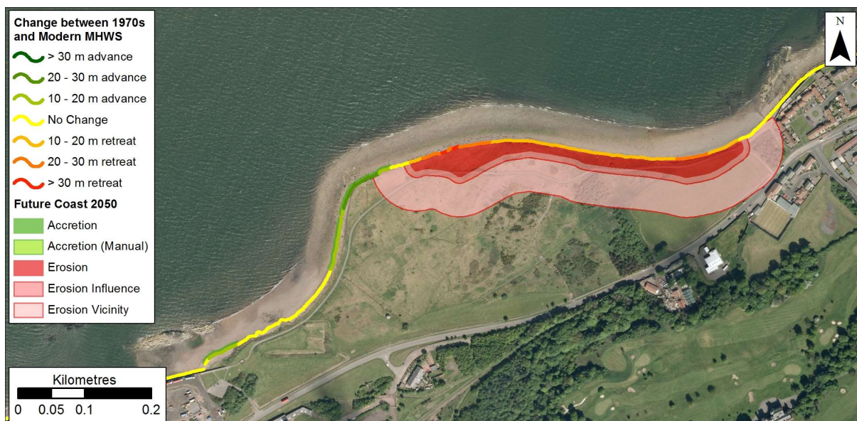
Figure 1.18: Possible future coastline position in 2050 based on rates between 1970 and Modern MHWS data east of Prestonpans. Getmapping are our current providers of Scotland-wide digital aerial imagery© Getmapping plc.
