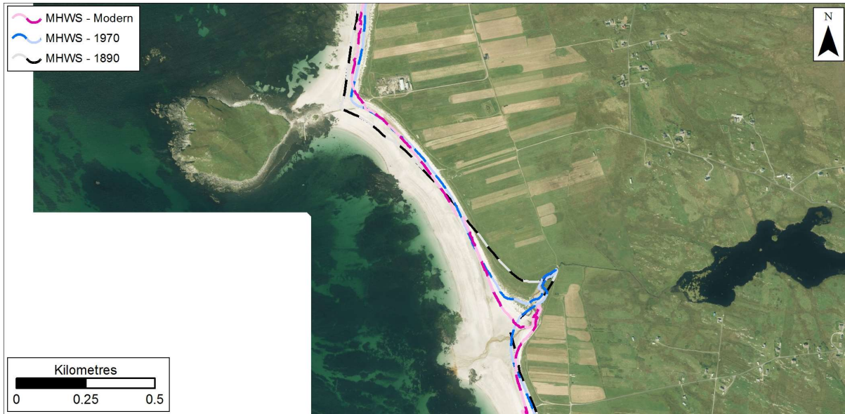
Figure 9.33: MHWS position in 1890, 1970s, and Modern datasets at North Boisdale. Getmapping are our current providers of Scotland-wide digital aerial imagery© Getmapping plc.
