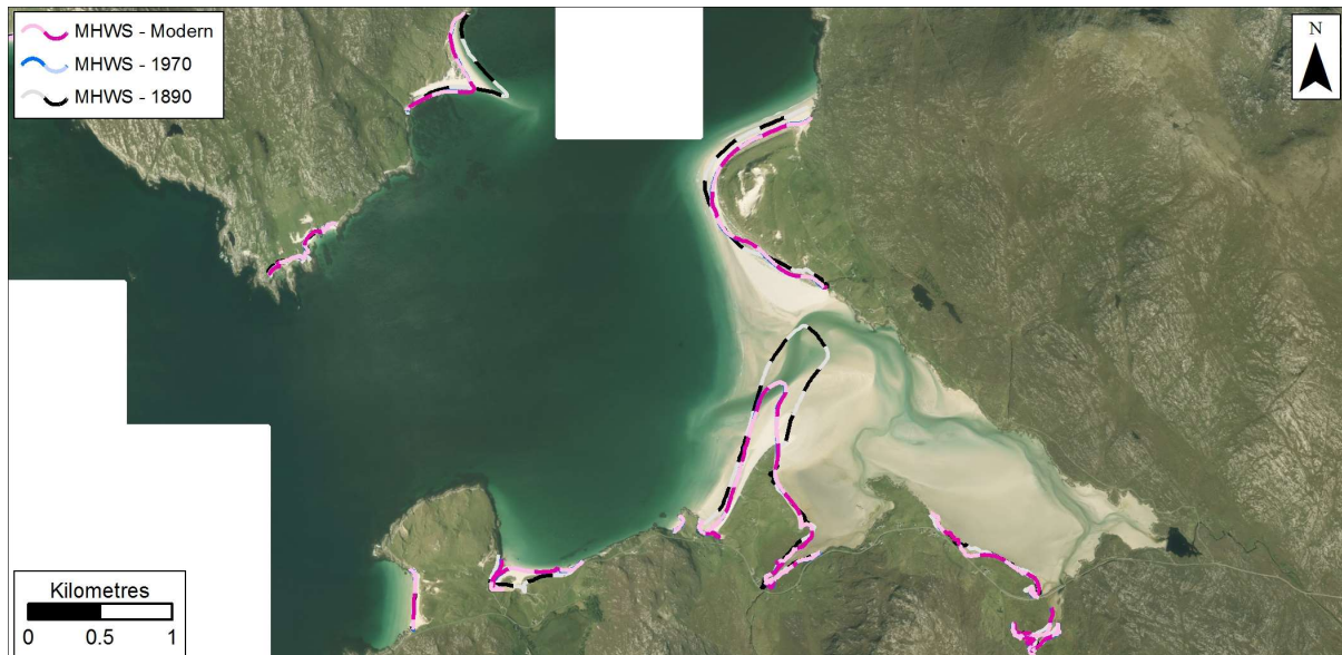
Figure 9.3: MHWS position in 1890, 1970s, and Modern datasets at Luskentyre and Taransay. Getmapping are our current providers of Scotland-wide digital aerial imagery© Getmapping plc.
