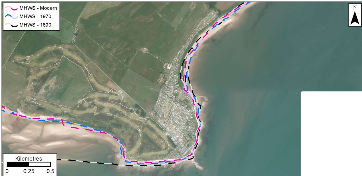
Figure 7.13: MHWS position in 1890, 1970s, and Modern datasets at Carsethorn. Getmapping are our current providers of Scotland-wide digital aerial imagery© Getmapping plc.
