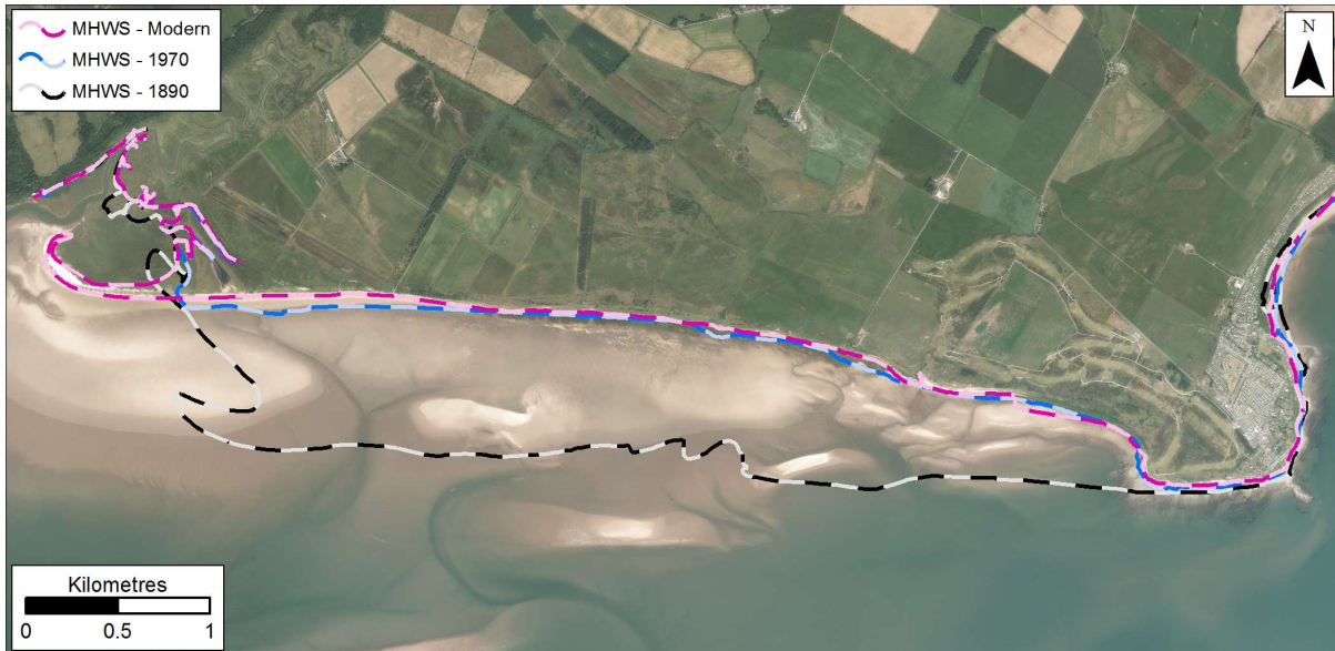
Figure 7.11: MHWs position in 1890, 1970s, and Modern datasets from Mersehead Sands to Southerness. Getmapping are our current providers of Scotland-wide digital aerial imagery© Getmapping plc.
