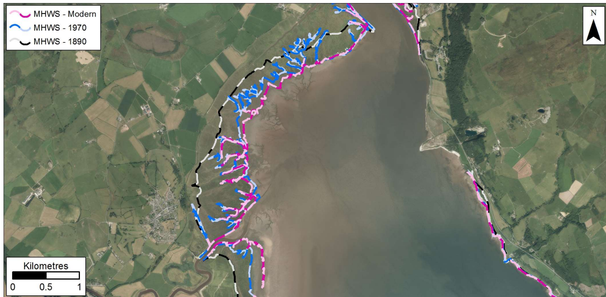
Figure 7.6: MHWS position in 1890, 1970s, and Modern datasets at Wigtown. Getmapping are our current providers of Scotland-wide digital aerial imagery© Getmapping plc.
