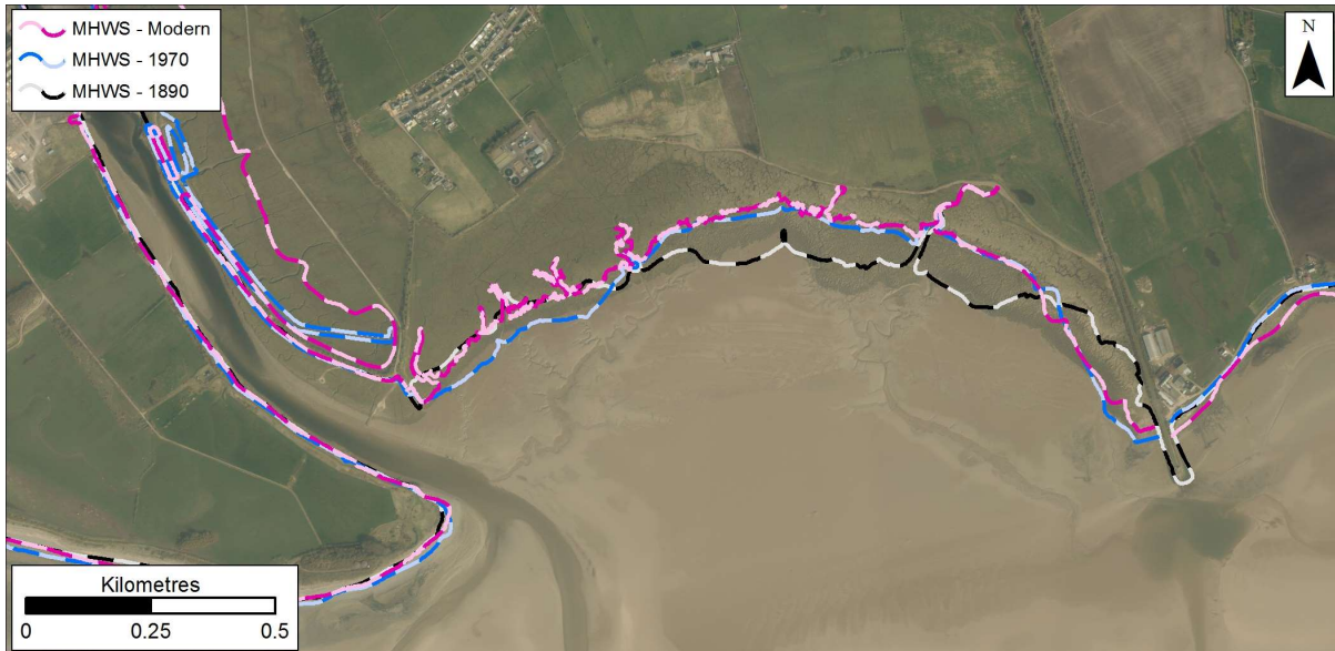
Figure 7.20: MHWS position in 1890, 1970s, and Modern datasets at east of the Annan mouth. Getmapping are our current providers of Scotland-wide digital aerial imagery © Getmapping plc.
