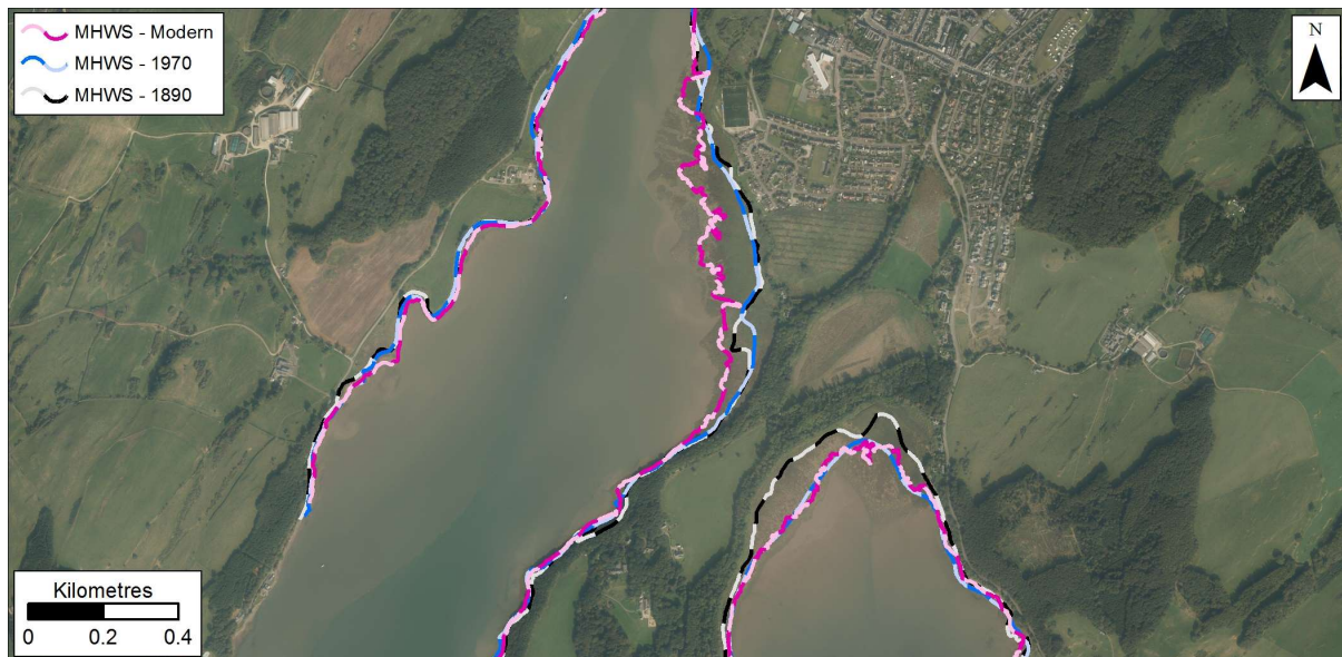
Figure 7.10: MHWs position in 1890, 1970s, and Modern datasets at Kirkcubright. Getmapping are our current providers of Scotland-wide digital aerial imagery © Getmapping plc.
