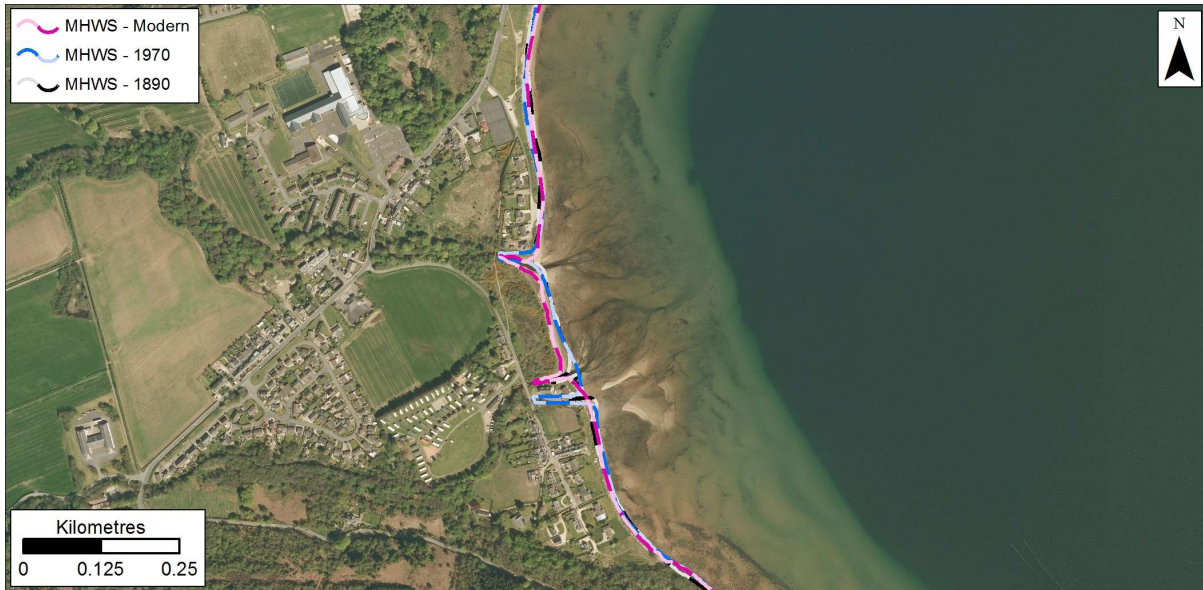
Figure 6.10: MHWS position in 1890, 1970s, and Modern datasets at Lamlash. Getmapping are our current providers of Scotland-wide digital aerial imagery© Getmapping plc.
