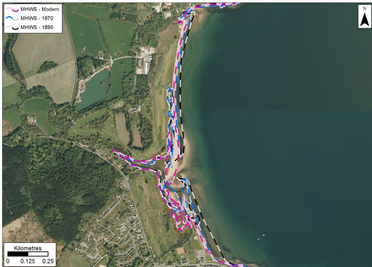
Figure 6.8: MHWS position in 1890, 1970s, and Modern datasets at Brodick Bay. Getmapping are our current providers of Scotland-wide digital aerial imagery © Getmapping plc.
