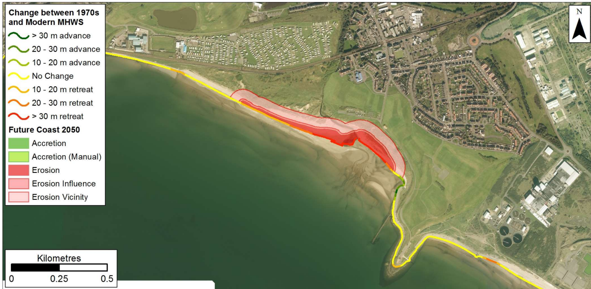
Figure 6.32: Possible future coastline position in 2050 based on rates between 1970 and Modern MHWS data at Saltcoats. Getmapping are our current providers of Scotland-wide digital aerial imagery© Getmapping plc.
