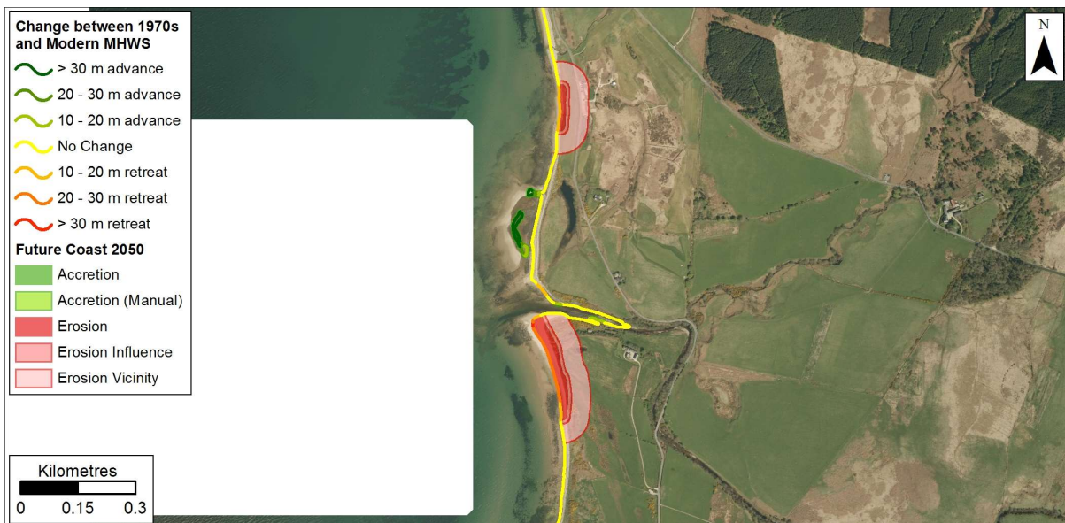
Figure 6.13: Possible future coastline position in 2050 based on rates between 1970 and Modern MHWS data at Machrie. Getmapping are our current providers of Scotland-wide digital aerial imagery© Getmapping plc.
