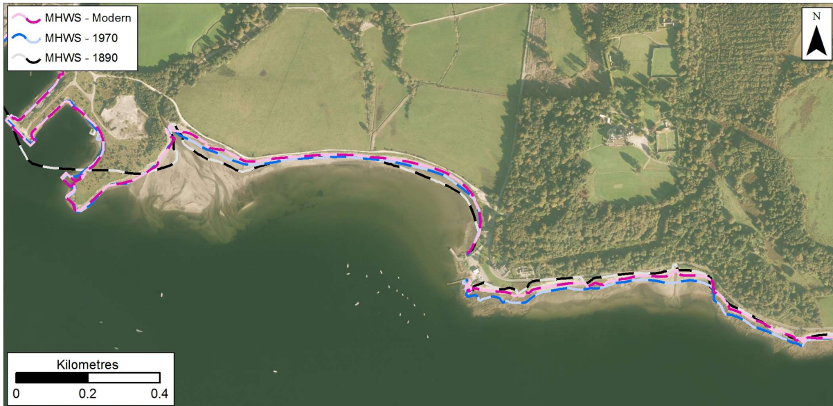
Figure 6.17: MHWs position in 1890, 1970s, and Modern datasets. Getmapping are our current providers of Scotland-wide digital aerial imagery© Getmapping plc.
