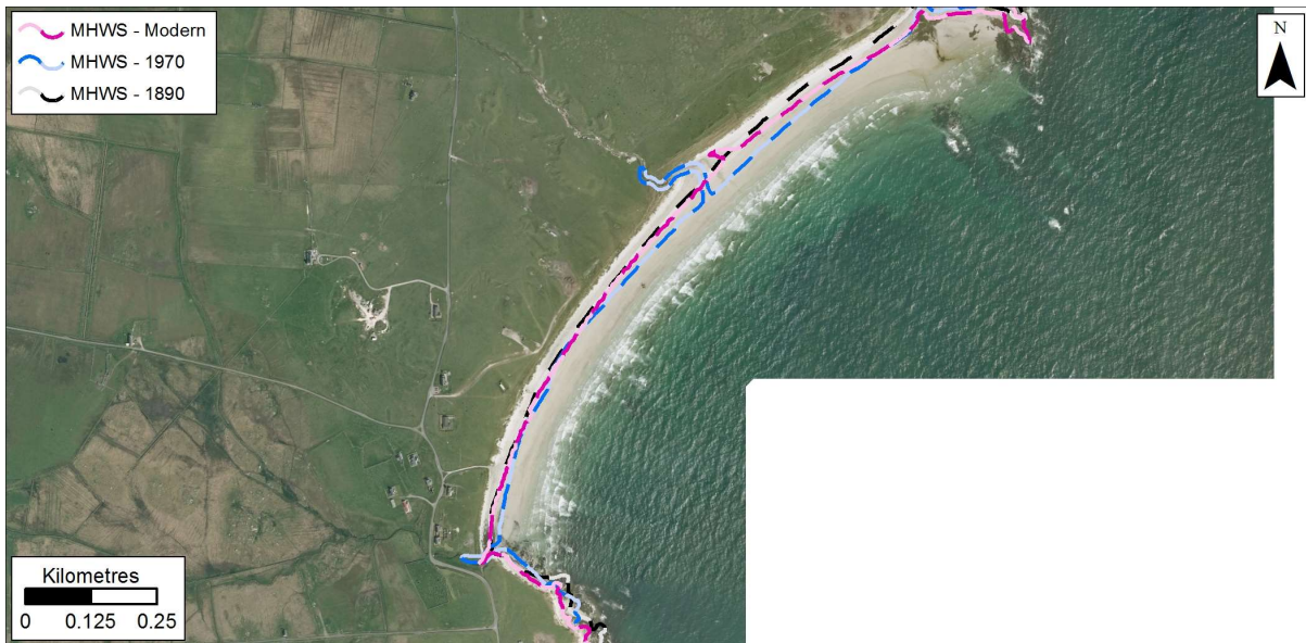
Figure 5.41: MHWS position in 1890, 1970s, and Modern datasets at Traigh Shorobaidh. Getmapping are our current providers of Scotland-wide digital aerial imagery© Getmapping plc.
