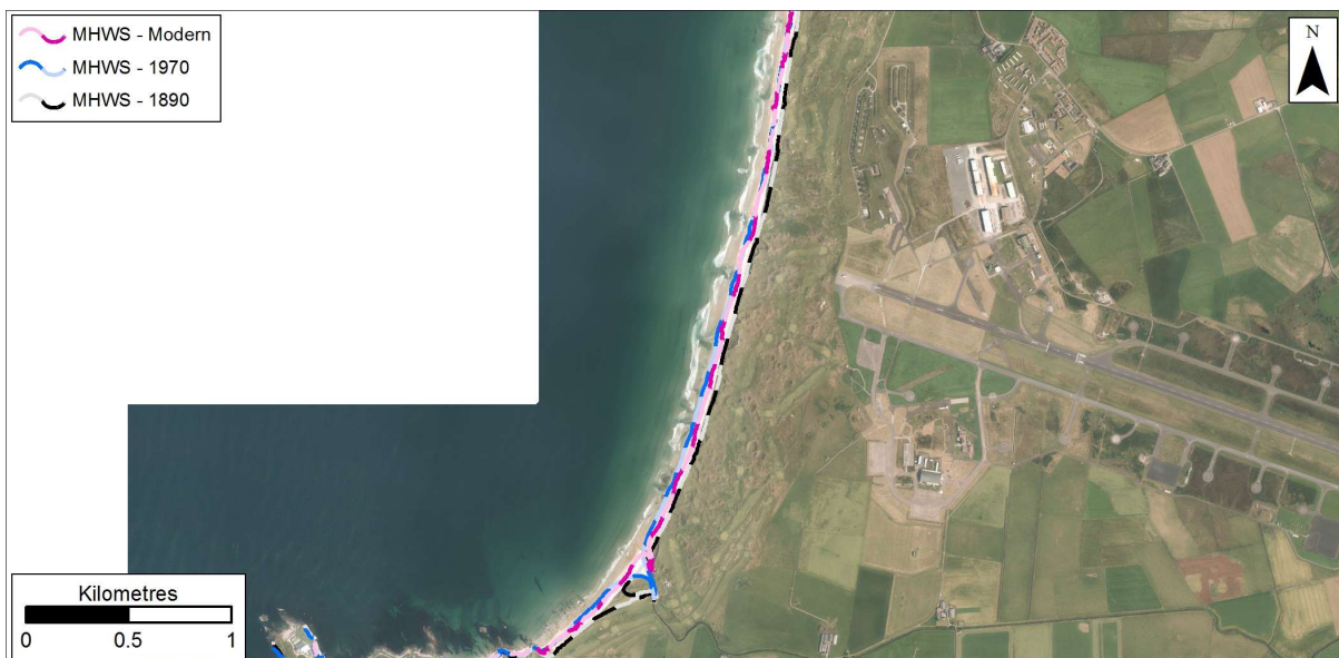
Figure 5.23: MHWS position in 1890, 1970s, and Modern datasets at Machrihanish. Getmapping are our current providers of Scotland-wide digital aerial imagery© Getmapping plc.
