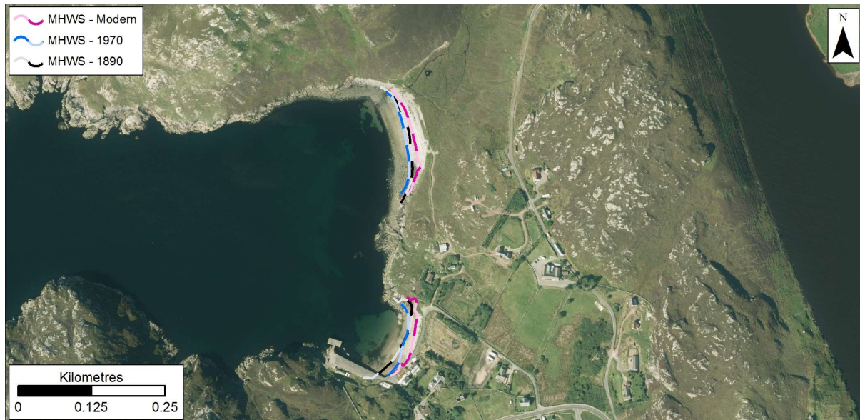
Figure 5.3: MHWS position in 1890, 1970s, and Modern datasets at Kinlochbervie. Getmapping are our current providers of Scotland-wide digital aerial imagery© Getmapping plc.
