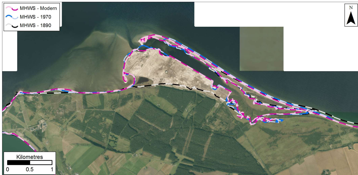
Figure 3.17: MHWS position in 1890, 1970s, and Modern datasets at Whiteness Head. Getmapping are our current providers of Scotland-wide digital aerial imagery © Getmapping plc.
