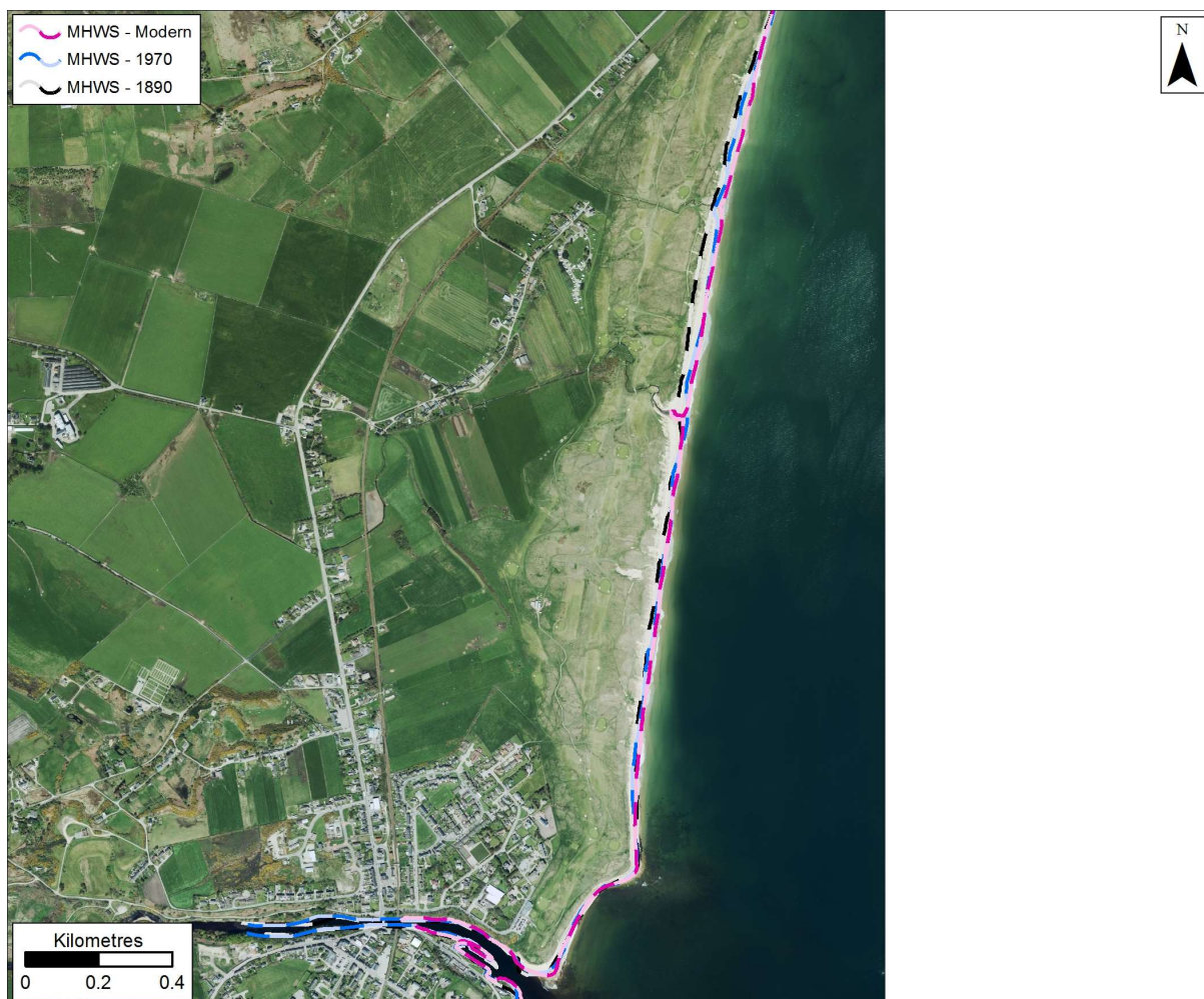
Figure 3.35: MHWS position in 1890, 1970s, and Modern datasets at Brora. Getmapping are our current providers of Scotland-wide digital aerial imagery© Getmapping plc.
