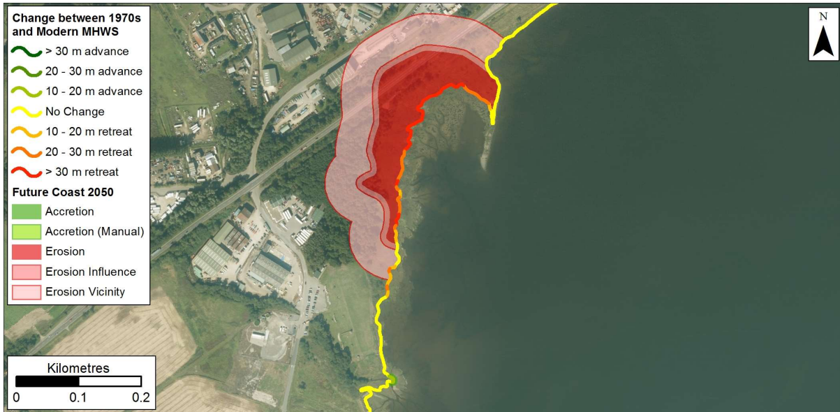
Figure 3.22: Possible future coastline position in 2050 based on rates between 1970 and Modern MHWS data near Culcairn in the Cromarty Firth. Getmapping are our current providers of Scotland-wide digital aerial imagery© Getmapping plc.
