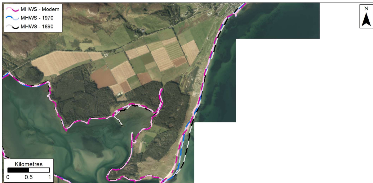
Figure 3.30: MHWS position in 1890, 1970s, and Modern datasets at Golspie. Getmapping are our current providers of Scotland-wide digital aerial imagery © Getmapping plc.
