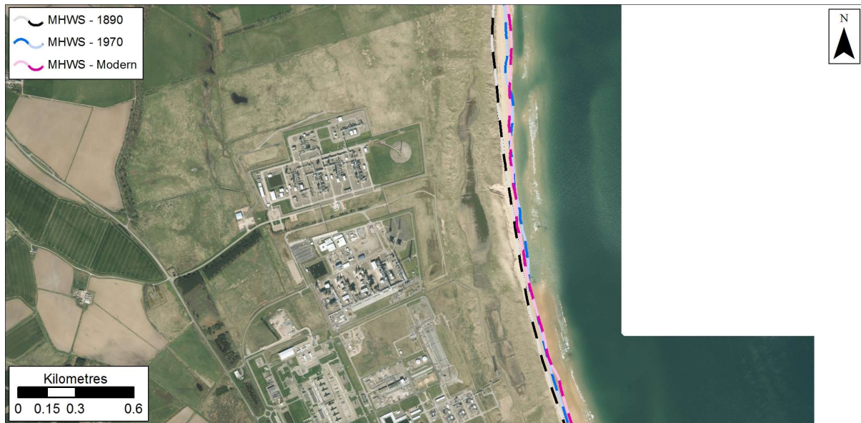
Figure 2.32: MHWS position in 1890, 1970s, and Modern datasets at the St. Fergus Gas Terminal. Getmapping are our current providers of Scotland-wide digital aerial imagery© Getmapping plc.
