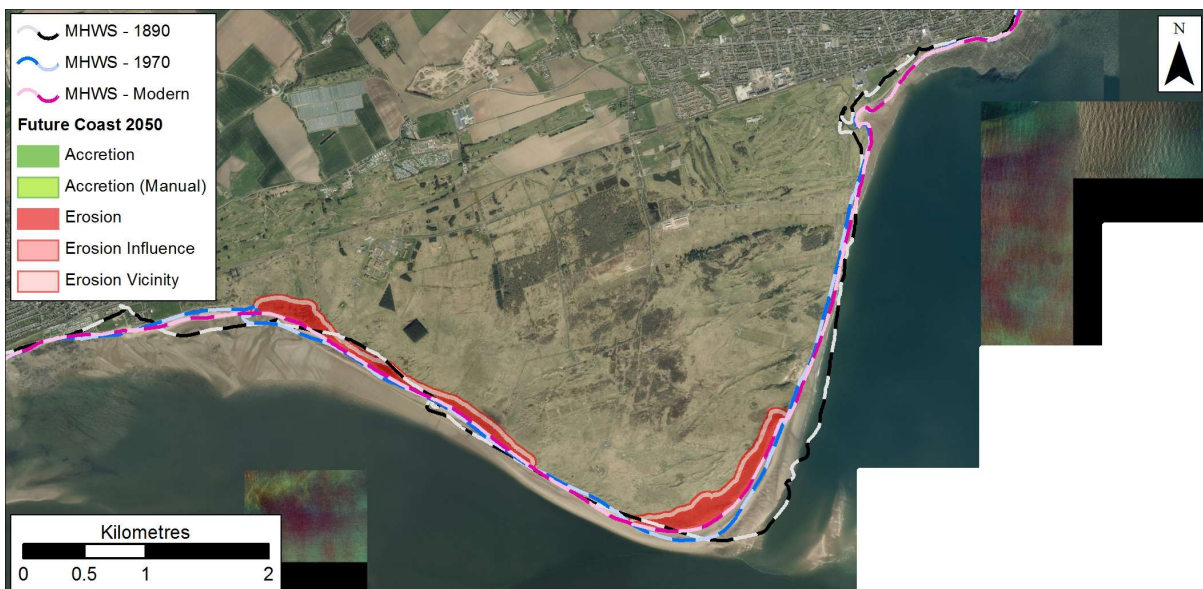
Figure 2.18: Possible future coastline position in 2050 based on rates between 1970 and Modern MHWS data at Barry Links. Getmapping are our current providers of Scotland-wide digital aerial imagery© Getmapping plc.
