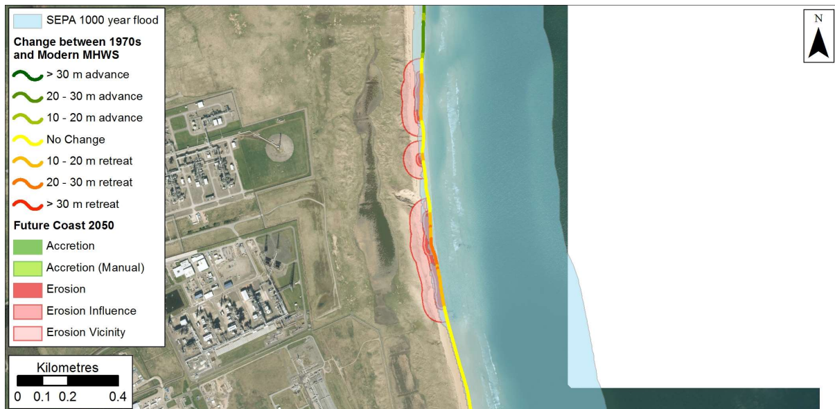
Figure 2.33: Possible future coastline position in 2050 based on rates between 1970 and Modern MHWS data with the SEPA 1000 year flood envelope at St. Fergus Gas Terminal. Getmapping are our current providers of Scotland-wide digital aerial imagery© Getmapping plc.
