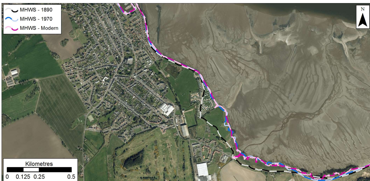
Figure 2.11: MHWS position in 1890, 1970s, and Modern datasets at Tayport. Getmapping are our current providers of Scotland-wide digital aerial imagery© Getmapping plc.
