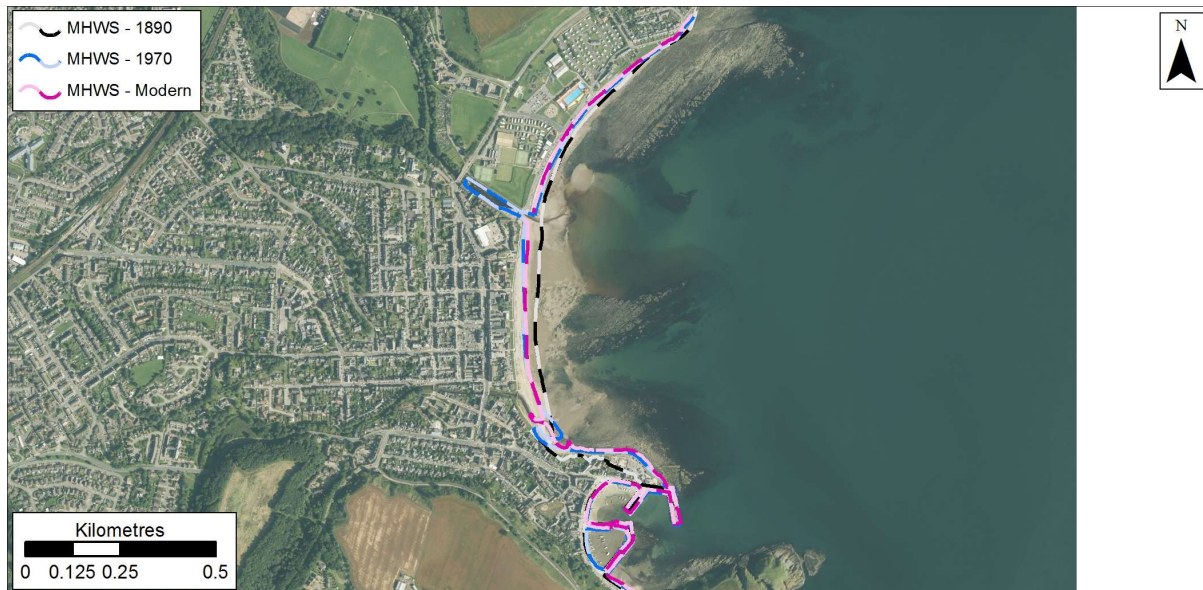
Figure 2.21: MHWS position in 1890, 1970s, and Modern datasets at Stonehaven. Getmapping are our current providers of Scotland-wide digital aerial imagery© Getmapping plc.
