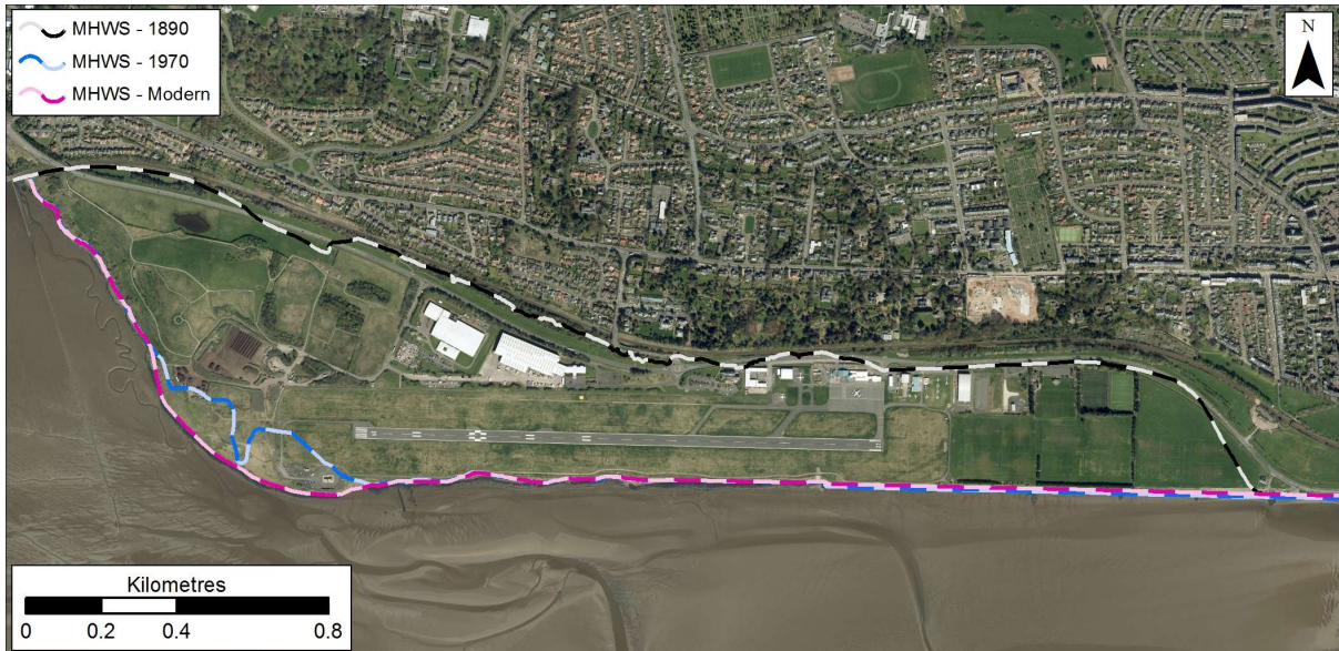
Figure 2.13: MHWS position in 1890, 1970s, and Modern datasets at Dundee Airport. Getmapping are our current providers of Scotland-wide digital aerial imagery © Getmapping plc.
