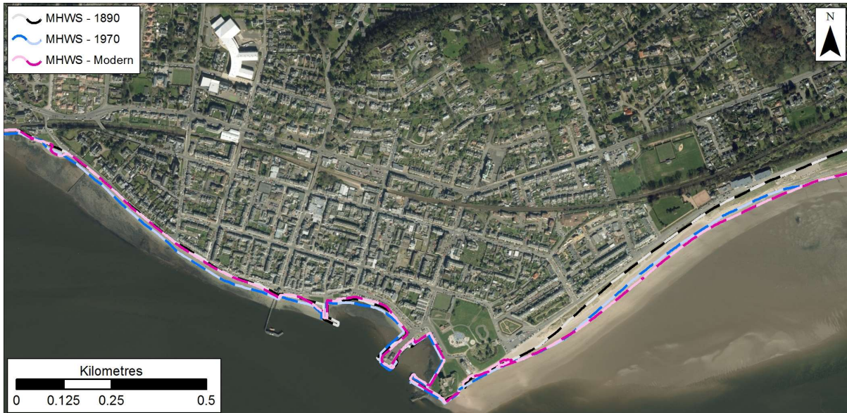
Figure 2.14: MHWS position in 1890, 1970s, and Modern datasets at Broughty Ferry. Getmapping are our current providers of Scotland-wide digital aerial imagery© Getmapping plc.
