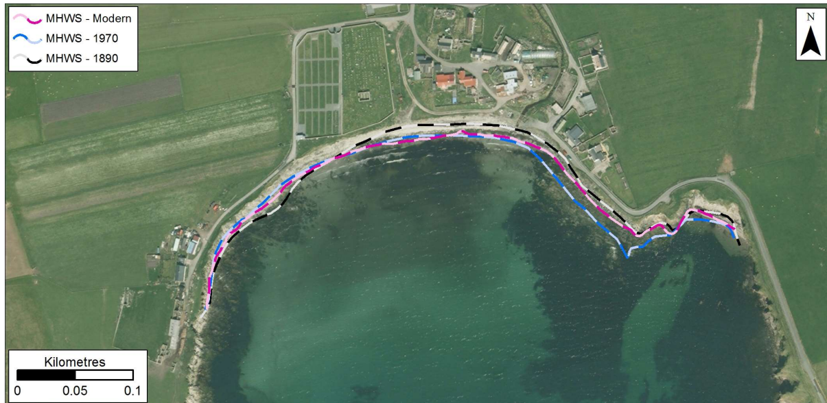
Figure 11.3: MHWS position in 1890, 1970s, and Modern datasets at Sandwick. Getmapping are our current providers of Scotland-wide digital aerial imagery© Getmapping plc.
