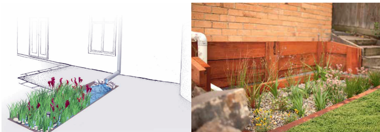
Figure B1.18. Inground raingardens. Guidance schematic (left) and property level installation (right). Image source: Melbourne Water.
