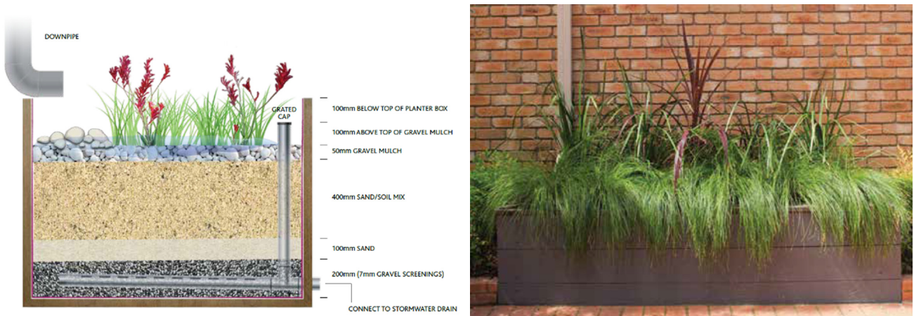
Figure B1.16. Boxed raingardens. Guidance schematic (left) and property level installation (right). Image source: Melbourne Water.
