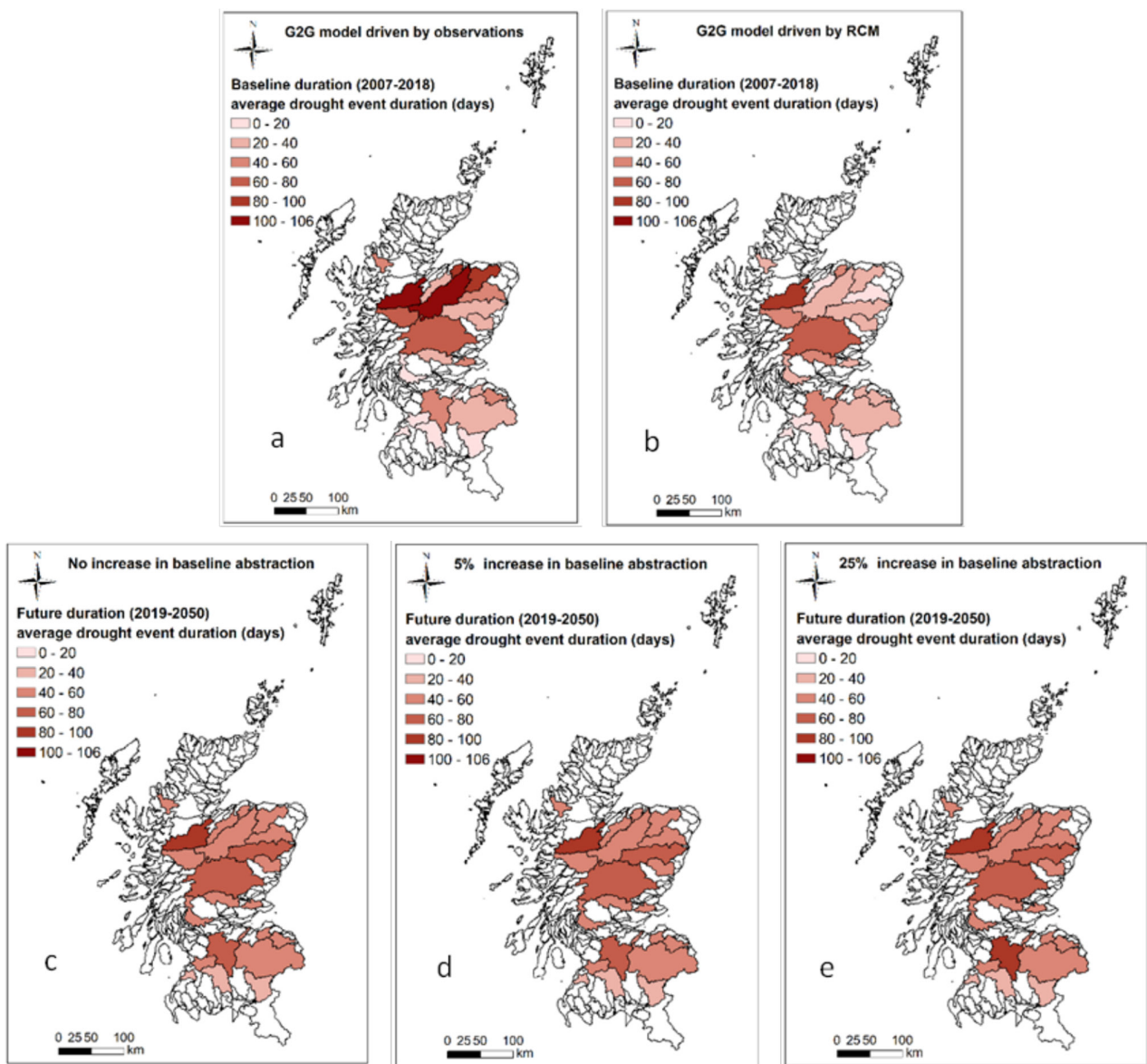
Figure 7: Average drought duration (in days) extracted from the drought profiling framework for the (a) historical period (2007–2018) driven by G2G model simulated flows using observations and baseline abstractions (b) historical period (2007–2018) driven by G2G model simulated flows using RCM and baseline abstractions (c) future (2019–2050) using G2G projected flows and baseline abstractions. (d) future period (2019–2050) using G2G projected flows and 5% increase in baseline abstractions. (e) future (2019–2050) using G2G projected flows and 25% increase in baseline abstractions. Catchments in white were not included in the analysis due to lack of data.
