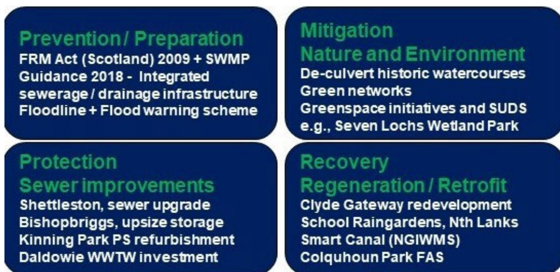
Figure 6: Types of FRM measures implemented by the MGSDP and Partners (after Wesselink et al. 2015).
