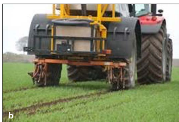
Figure 4. Photographs of a) the new EVOBIB and b) the older XEOBIB tyres. Note the block shapes in the centre of the tread in the new EVOBIB tyre and the spiked harrow used alongside the XEOBIB tyre for loosening the soil (courtesy of B. McKenzie).
