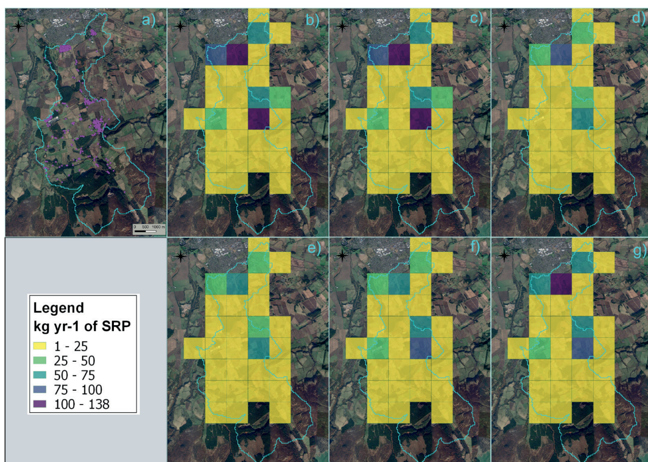
Figure 8. A comparison of simulated SRP losses from STS in the Linkwood Burn catchment a) modelled location of STS, b) baseline scenario, c) all STS fitted with primary treatment, d) all STS fitted with secondary treatment, e) all STS fitted with tertiary treatment, f) no STS directly connected to streams and g) all STS well maintained.
