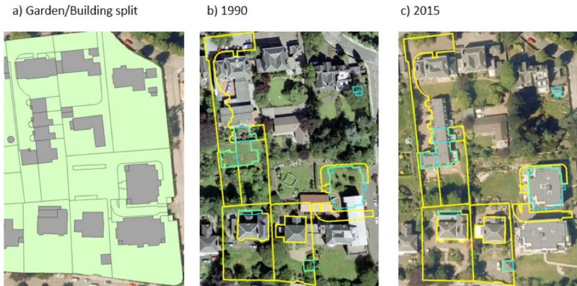
Figure 13 Identifying increased urban area in garden and building polygons. a) Shows the current building and garden split; b) shows the aerial photo in 1990, c) shows the aerial photo in 2015. Yellow polygons are garden polygons showing a significant increase in urban area between 1990 and 2015. Blue polygons are building polygons showing a significant increase in urban area between 1990 and 2015.
