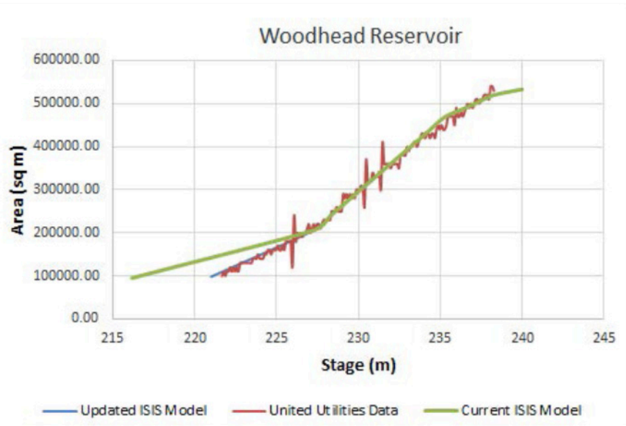
Figure A4.3.2 Comparison between current (green) and updated (blue) stage-area curves for FM (ISIS) models and United Utilities data (red) for Woodhead Reservoir. (Source: CH2M (2016))
