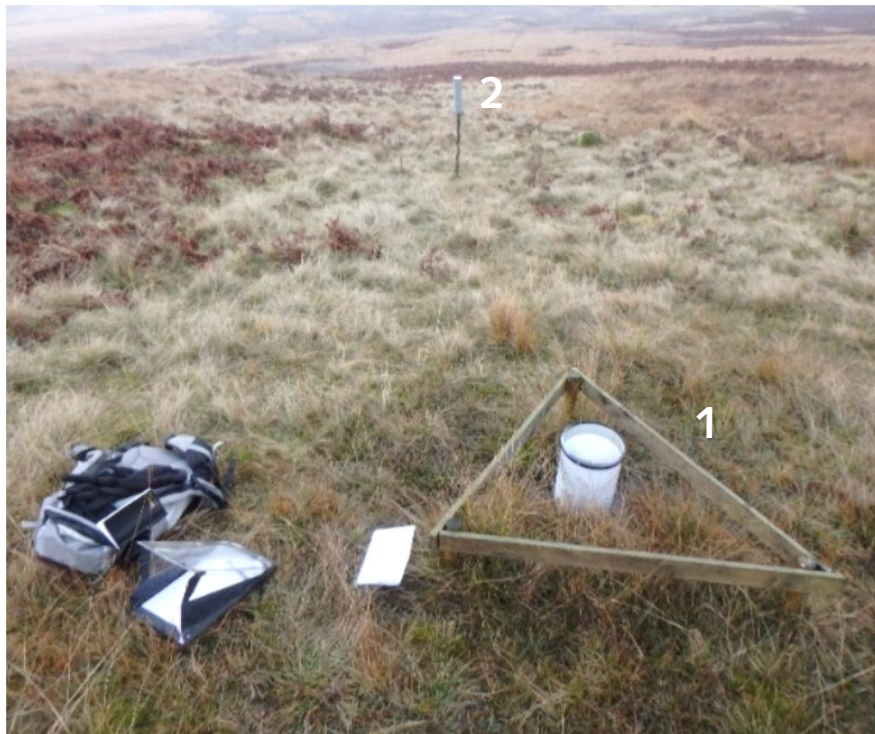
Figure 1. A Topography, sub-catchments and monitoring network of the River Knaik catchment. B A tipping bucket rainfall gauge (1) linked by a buried cable to a combined data logger and telemetry aerial (2) to enable remote data collection, in the Corriebeagh Burn sub-catchment.
